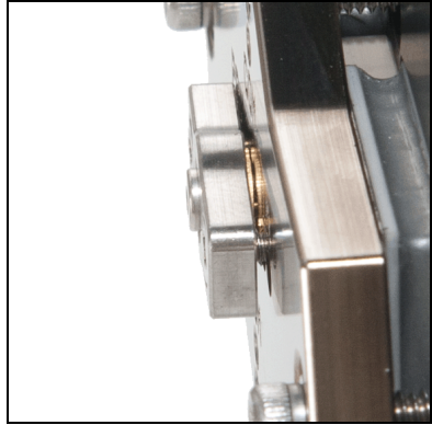
BAD: Diode improperly clamped, clip is uneven with cold plate
