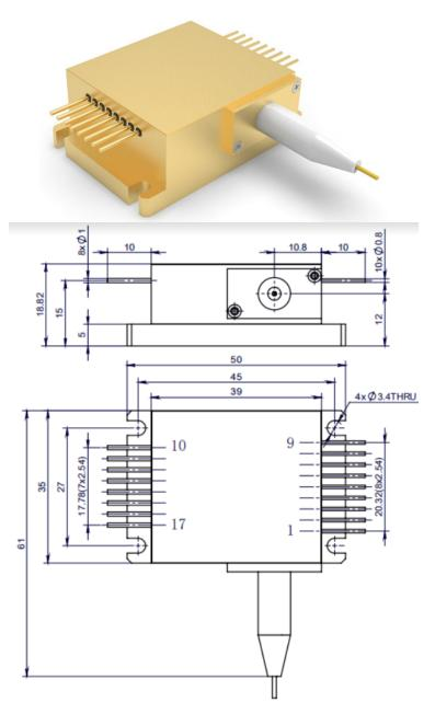
The table below shows the dimensions and the pin numbers of the new 2CM/4CM package.
